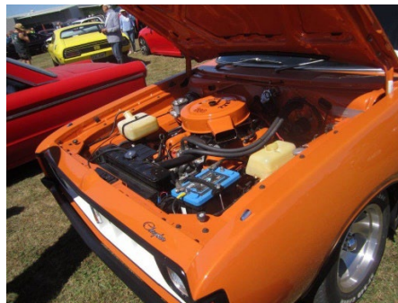
A beautiful engine bay in a 1975 VK Charger E57 showing off the 360ci V8 to brilliant effect.
